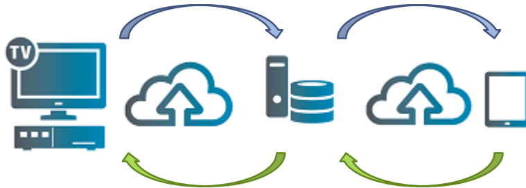
Figure 2: ConnectTV functionality: Remote user control of the STB and streaming of content to the remote user outside of the home network across the internet.
